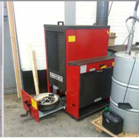
Built-in overflow protection for burner dish.
